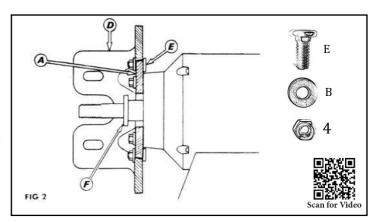
Fit the Main Bracket (D) using flat head clamp bolts (E) through the 3 slots (Fig 1: C) in outer edge of the adaptor plate, with flat heads of bolt facing the grinder. With angle face of bracket approximately vertical, tighten  $\frac{1}{4}$ " nuts (4) evenly. The adaptor plate should be flush with the main bracket. If the Multitool is to be used in a vertical position simply loosen nuts, tap main bracket (D) to loosen. Swivel to desired position and retighten nuts (4).
