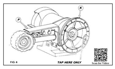
Fit the Drive Pulley (K) by sliding over the shaft of the grinder. Fit tightly against the flange. Use  $\frac{1}{2}$ " or  $\frac{5}{4}$ " diameter washer (Fig 3. F ) under the nut and tighten with a socket spanner. If disc face does not run true, tap gently on the inside edge of rim only.
