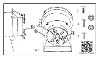
From the right hand end of the grinder, remove wheel cover, wheel, wheel flanges and wheel guard. Fit slotted adaptor plate (A) using either  $\frac{1}{4}$ " bolt (1), 5mm Bolt (2) or  $\frac{3}{16}$ " Bolt (3) provided. Use appropriate size washers under heads (B). The outer edge of the adaptor plate is tapered. Face smallest side of taper away from grinder as shown in Fig 1. (A)
