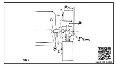
Idler arm Cam plate (M) must now be set  $\frac{1}{4}$ " (6mm) clear of inside edge of the drive pulley (Fig 4. K) Slots are provided under  $\frac{5}{16}$ " bolts (Fig 3. J) for this adjustment.
